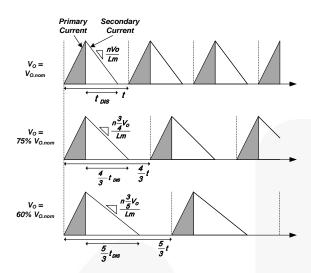
Figure 18. Primary and Secondary Current
