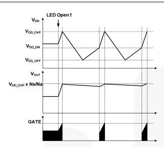
Figure 22. Waveforms at Open-LED Condition
