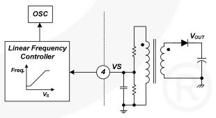
Figure 17. Linear Frequency Control
