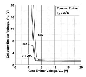
Figure 7. Saturation Voltage vs. V<sub>GE</sub>
