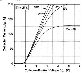
Figure 3. Typical Saturation Voltage Characteristics
