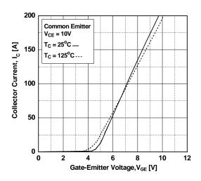
Figure 6. Saturation Voltage vs. V<sub>GE</sub>
