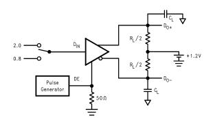
Figure 6. Driver TRI-STATE Delay Test Circuit
