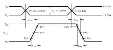
Figure 9. Receiver Propagation Delay and Transition Time Waveforms
