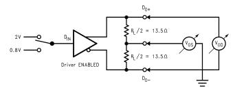
Figure 3. Differential Driver DC Test Circuit
