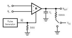
Figure 10. Receiver TRI-STATE Delay Test Circuit
