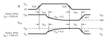
Figure 11. Receiver TRI-STATE Delay Waveforms
