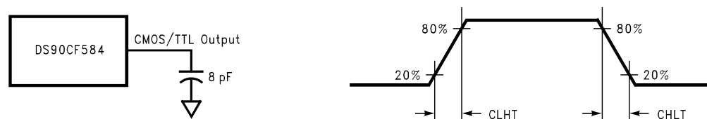
Figure 6. DS90CF584 (Receiver) CMOS/TTL Output Load and Transition Times
