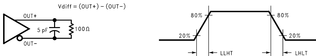
Figure 5. DS90CF583 (Transmitter) LVDS Output Load and Transition Times
