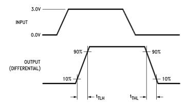
Input pulse; f = 1 MHz, 50%;  $t_r \le 6$  ns,  $t_f \le 6$  ns
