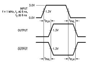
Figure 27. Propagation Delays
