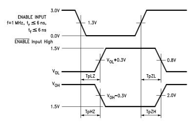
Figure 28. Enable and Disable Times
