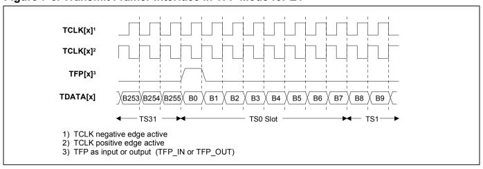
Figure 7-9. Transmit Framer Interface in Gapped-Clock Mode for E1
