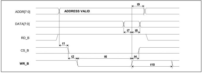
Figure 13-6. Motorola Bus Read Timing (BTS = 1/MUX = 0)
