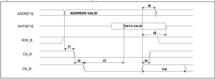
Figure 13-7. Motorola Bus Write Timing (BTS = 1/MUX = 0)
