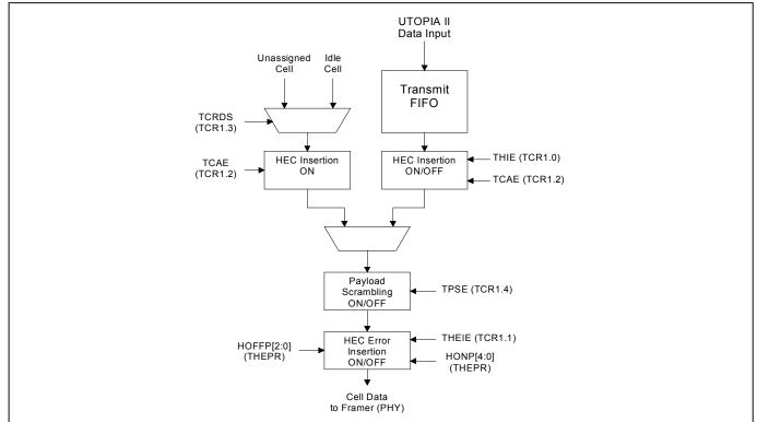
Figure 7-5. Transmit Cell Flow and Processing
