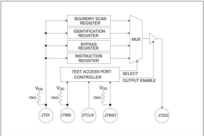
**TAP Controller State Machine.** The TAP controller is a finite state machine that responds to the logic level at JTMS on the rising edge of JTCLK (Figure 11-2).
