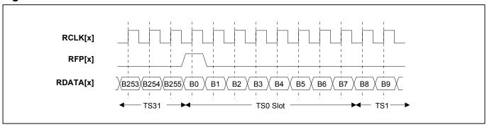
Figure 8-3. Receive Framer Interface in RFP Mode for E1
