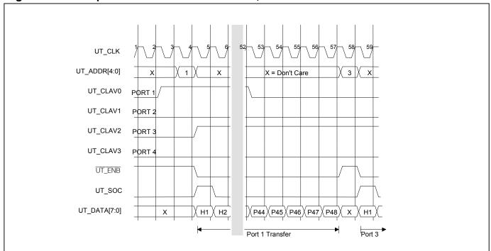
Figure 7-4. Example of Direct Status Indication, Transmit Direction
