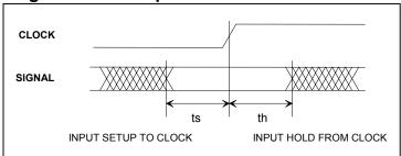
Figure 13-9. Delay Time Definition
