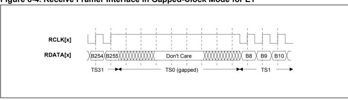
Figure 8-4. Receive Framer Interface in Gapped-Clock Mode for E1
