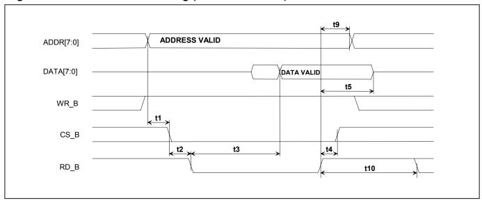
Figure 13-5. Intel Bus Write Timing (BTS = 0/MUX = 0)
