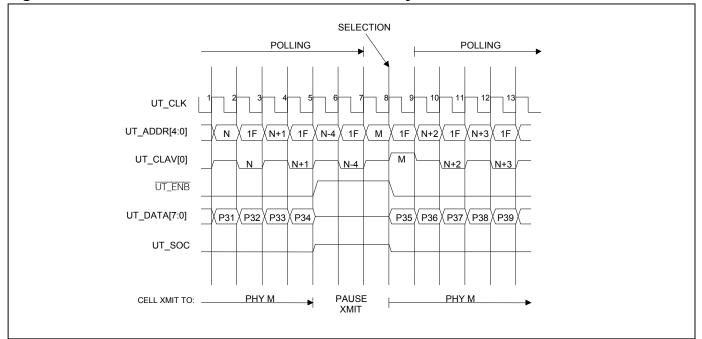
Figure 7-3. Transmission to PHY Paused for Three Cycles
