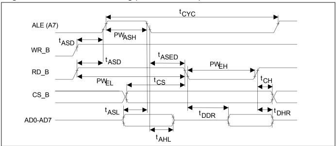
Figure 13-2. Intel Bus Write Timing (BTS = 0/MUX = 1)
