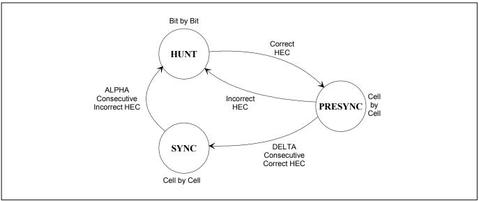
Figure 8-6. Header Correction State Machine
