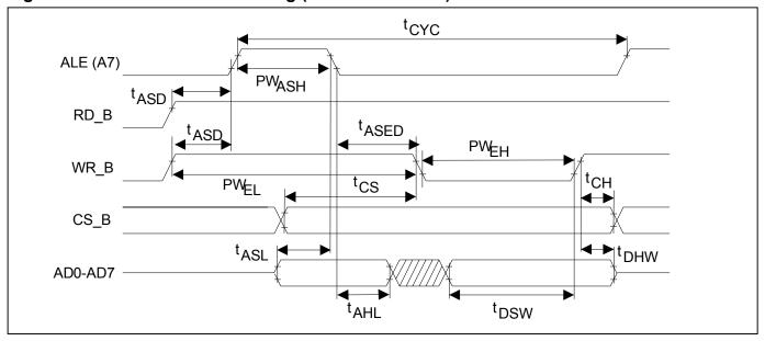
Figure 13-3. Motorola Bus Timing (BTS = 1/MUX = 1)
