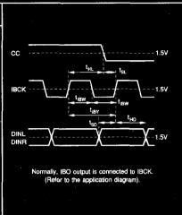
NOTE: (1) 3.232MHz = 64 x 50.5kHz (max sampling frequency).
