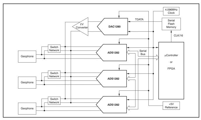
Figure 34. Three-Channel Seismic System Block Diagram
