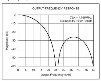
Figure 33. Output Frequency Response
