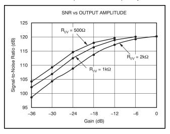
Figure 31. SNR vs Output Amplitude
