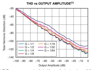
(1) THD measurement noise limited for amplitudes less than  $-10 \mbox{dB}.$
