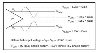
Figure 28. I/V Converter Output Voltage
