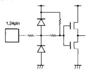
Input with pulldown resistors
