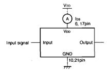
Fig. 4 Operating current measurement circuit
