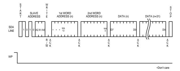
Fig.9 PAGE WRITE CYCLE TIMING
