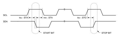
Fig.4 SYNCHRONOUS DATA TIMING
