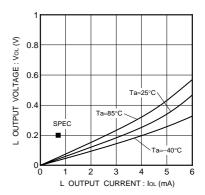
Fig.19 Low output voltage VoL-loL (Vcc=1.8V)
