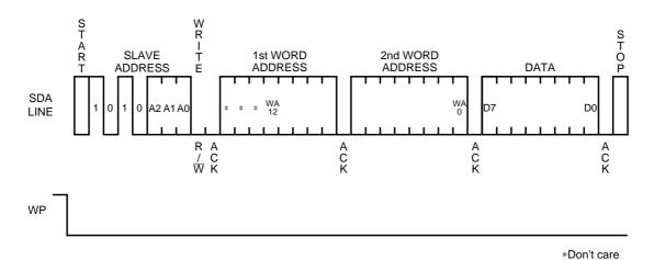
Fig.8 BYTE WRITE CYCLE TIMING
