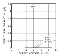
Fig.22 Output leakage current ILO(SDA)
