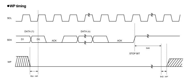
Fig.6(a) WP TIMING OF THE WRITE OPERATION
