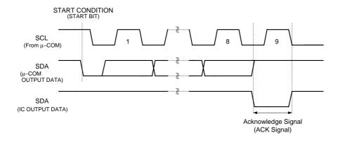
Fig.7 ACKNOWLEDGE RESPONSE FROM RECEIVER
