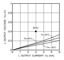
Fig.20 Low output voltage VoL-loL (Vcc=2.5V)
