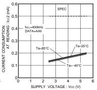
Fig.24 Read operating current Icc2 (fscL=400kHz)
