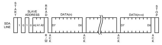
Fig.12 SEQUENTIAL READ CYCLE TIMING (Current Read)
