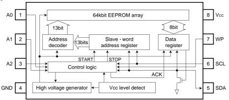
Fig.2 BLOCK DIAGRAM
