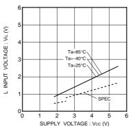
Fig.18 Low input voltage V<sub>IL</sub> (A0,A1,A2,SCL,SDA,WP)
