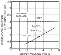
Fig.25 Write operating current Icc1 (fscL=100kHz)
