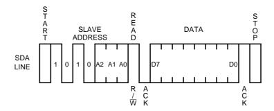
Fig.10 CURRENT READ CYCLE TIMING
