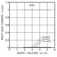
Fig.21 Input leakage current Iu (A0,A1,A2,SCL,WP)
