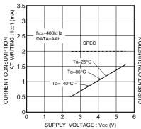
Fig.23 Write operating current Icc1 (fscL=400kHz)
