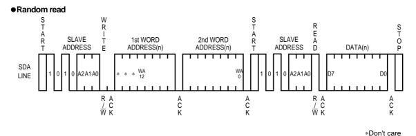
Fig.11 RANDOM READ CYCLE TIMING
