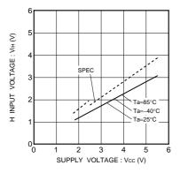
Fig.17 High input voltage V<sub>IH</sub> (A0,A1,A2,SCL,SDA,WP)
