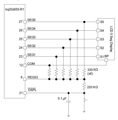
Figure 2. Typical LCD Implementation
