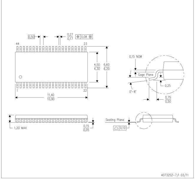
All linear dimensions are in millimeters. Dimensioning and tolerancing per ASME Y14.5M—1994. This drawing is subject to change without notice. NOTES:
