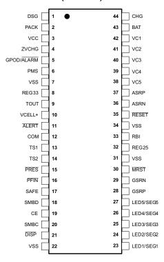
Figure 1. Package Pinout
