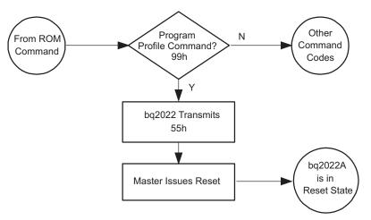
Figure 12. PROGRAM PROFILE Command Flow
