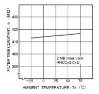
Fig. 6 Filter time constant (fo) vs. ambient temperature
