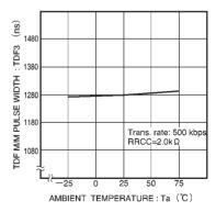
Fig. 8 TDF time constant vs. ambient temperature
