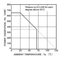
Fig. 3 Thermal derating characteristics
