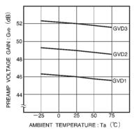
Fig. 4 Preamp voltage gain vs. ambient temperature
