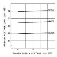
Fig. 5 Preamp voltage gain vs. power supply voltage
