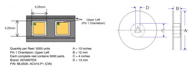
Figure 13. Package Orientation on Tape
