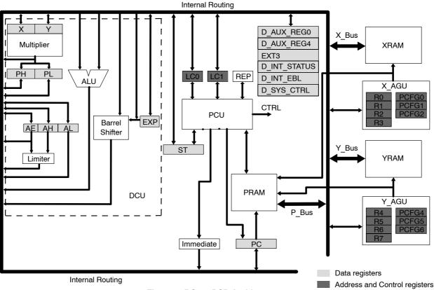
Figure 3. RCore DSP Architecture
