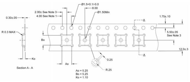
1. 10 sprockets hole pitch cumulative tolerance  $\pm 0.2$ .
