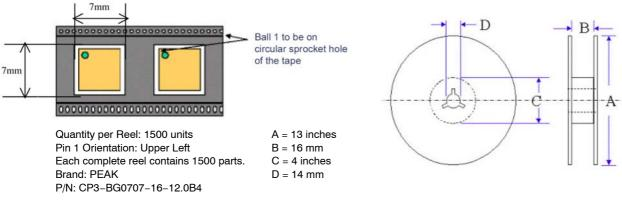
Figure 11. Package Orientation on Tape
