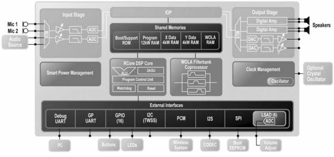
Figure 2. BELASIGNA 250 Architecture: A Complete Audio Processing System
