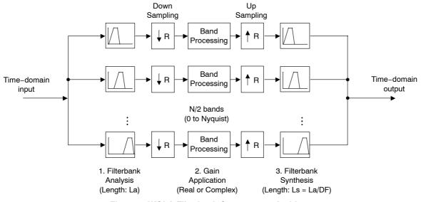
Figure 4. WOLA Filterbank Coprocessor Architecture
