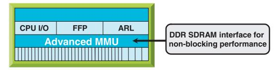
The **BCM5651** network switch is the most advanced multi-layer, singlechip solution for high density  $24 \times 10/100$  Mbps ports and  $4 \times 10/100/$ 1000 Mbps Ethernet uplinks.
