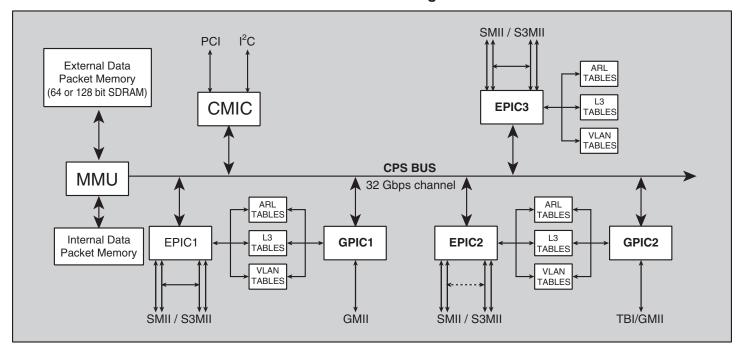
The **BCM5616**, with a forwarding rate of 6.6 Mpps, defines the next generation of performance for single-chip switching solutions. Through its advanced ContentAware<sup>TM</sup> feature set, the StrataSwitch II<sup>TM</sup> product family supports advanced applications and services, at wire speed, with nonblocking performance.
