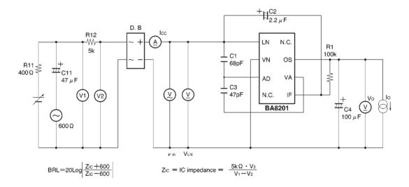
Fig. 3 Measurement circuit (3)
