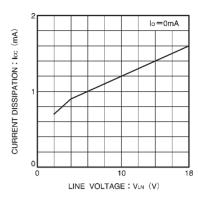
Fig. 7 Current dissipation vs. line voltage
