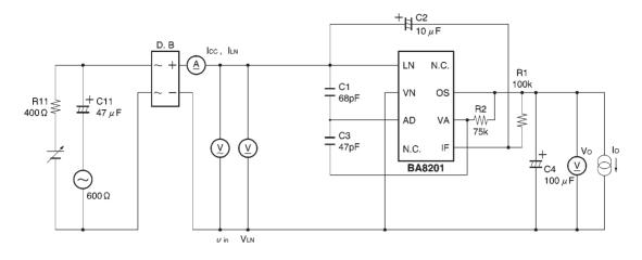
Fig. 2 Measurement circuit (2)
