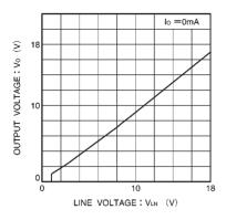
Fig. 5 Output voltage vs. line voltage (without R2)
