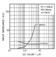
Fig. 9 LN input impedance vs. C2
