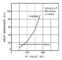
Fig. 8 LN input impedance vs. R1
