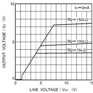
Fig. 6 Output voltage vs. line voltage (with R2)
