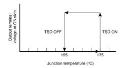
TSD ON (Typ. : 175°C) All output transistor OFF.
