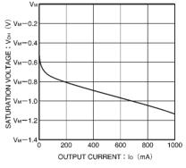
Fig.19 Upper-side output saturation voltage vs. output current
