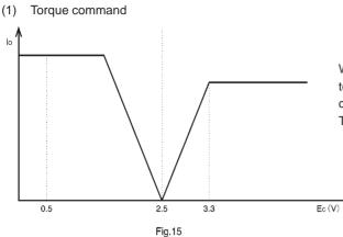
When operating with  $E_{CR} = 2.5V$ , the voltage range for the torque command input is 0.5V to 3.3V, and therefore, the characteristic will be unbalanced as shown in Fig.15. Take due care.
