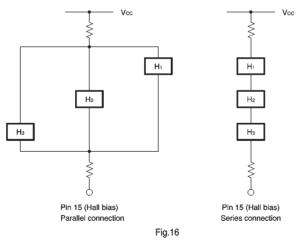
Set the Hall input voltage in the range 1.0V to 4.0V.
