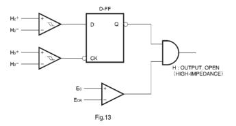
The reverse detection circuit construction is shown in Fig.13.
