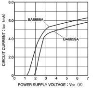
Fig.18 Power supply current vs. power supply voltage
