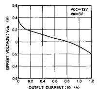
Fig.11 Offset voltage vs. output current
