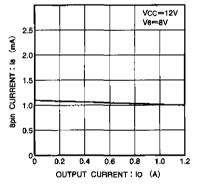
Fig.12 Pin-6 current vs. output current
