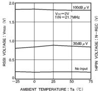
Fig. 13 RSSI voltage vs. ambient temperature
