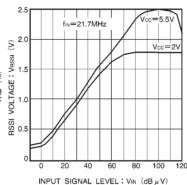
Fig. 11 RSSI voltage vs. input signal level
