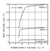
Fig. 12 RSSI voltage vs. power supply voltage
