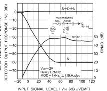
Fig. 15 Detector output response,
