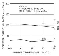
Fig. 10 Detector output level, THD vs. ambient temperature
