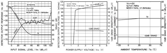
Fig. 7 Detector output response, AMR, SINAD vs. input signal leve
