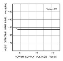
Fig. 4 Song detection input level 1 vs. power supply voltage
