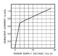
Fig. 3 Quiescent current vs. power supply voltage
