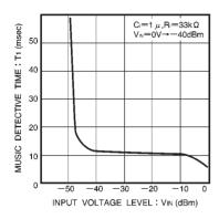
Fig. 6 Song detection time vs. input voltage level
