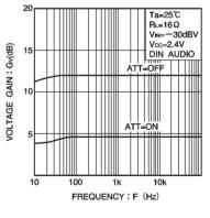
Fig.7 Voltage gain vs. frequency
