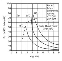
Fig.4 Maximum allowable power output per channel  $(P_{0} (MAX.) / ch)$  vs. supply voltage (V<sub>cc</sub>)
