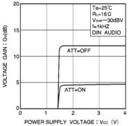
Fig.6 Voltage gain vs. power supply voltage
