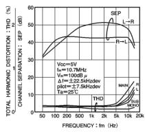
Fig. 6 Channel separation and THD vs. frequency
