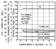
Fig. 8 AM characteristics vs. power suppy voltage
