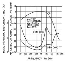
Fig. 9 AM detector output and THD vs. frequency
