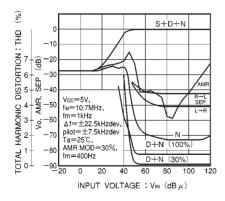
Fig. 3 FM input/output characteristics
