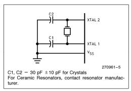
**Figure 4. Oscillator Connections**
