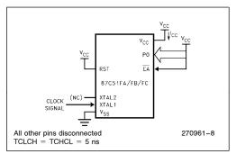
Figure 7. I<sub>CC</sub> Test Condition, Active Mode
