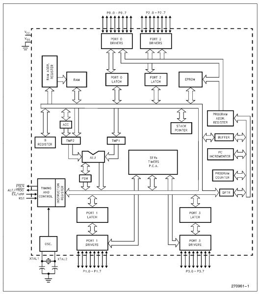
Figure 1. 87C51FB/FC Block Diagram
