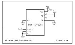
Figure 9. I<sub>CC</sub> Test Condition, Power Down Mode.  $V_{CC} = 2.0V$  to 5.5V.
