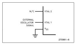
Figure 5. External Clock Drive Configuration
