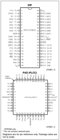
Figure 3. Pin Connections (Top View)
