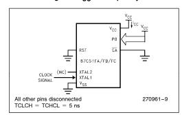
Figure 8. I<sub>CC</sub> Test Condition Idle Mode
