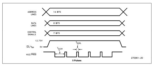
Figure 12. Programming Signal's Waveforms
