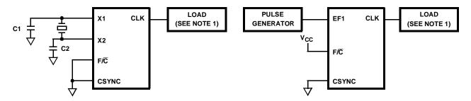
FIGURE 6. TCHCL, TCLCH LOAD CIRCUITS
