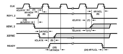
FIGURE 3. WAVEFORMS FOR READY SIGNALS (FOR ASYNCHRONOUS DEVICES)
