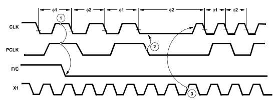
FIGURE 1A. F/C SWITCHED FROM HIGH (USING EFI INPUT) TO LOW (USING THE CRYSTAL INPUT X1)
