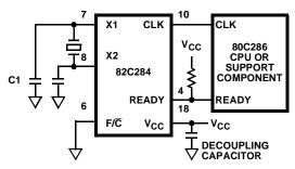
FIGURE 4. RECOMMENDED CRYSTAL AND READY CONDITIONS
