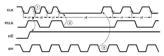
FIGURE 1B. F/C SWITCHED FROM LOW (USING THE CRYSTAL INPUT X1) TO HIGH (USING THE EFI INPUT)
