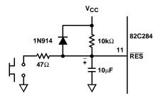
FIGURE 3. TYPICAL RC RES TIMING CIRCUIT
