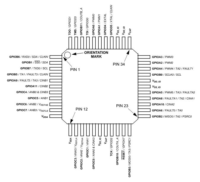
Figure 2. Top View, 56F8025 48-Pin LQFP Package
