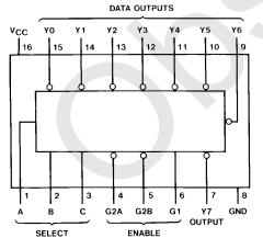
Order Number 54LS138DMQB, 54LS138FMQB, 54LS138LMQB, DM54LS138J, DM54LS138W, **DM74LS138M or DM74LS138N** See NS Package Number E20A, J16A, M16A, N16E or W16A
