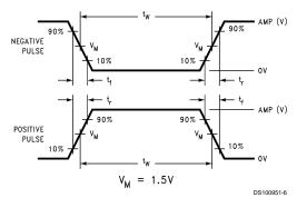
FIGURE 2. Test Input Signal Levels
