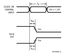
FIGURE 5. Propagation Delay, Pulse Width Waveforms
