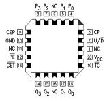
Figure 3. Pin Assignment for LCC
