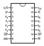
Figure 2. Pin Assignment for DIP and Flatpak
