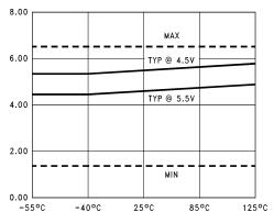
Figure 12.  $t_{PLZ}$ vs Temperature  $(T_A)$  $C_L = 50$  pF, 8 Outputs Switching
