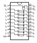
Figure 2. Pin Assignment
