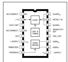
The A5354CA is a low-current, CMOS circuit providing all of the required features for an ionization-type smoke detector. A networking capability allows as many as 125 units to be interconnected so that if any unit senses smoke, all units will sound an alarm. In addition, special features are incorporated to facilitate alignment and test of the finished smoke detector. This device is designed to comply with Underwriters Laboratories Specification UL217.
