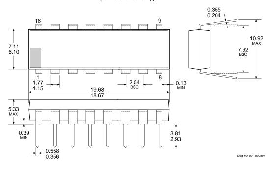
NOTES: 1. Lead thickness is measured at seating plane or below.
