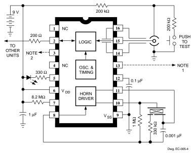
NOTE 1: An external resistor divider is used to adjust sensitivity for the particular smoke chamber.
