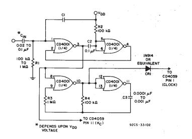
For changing from any mode other than mode 5 (with power on), apply positive pulse to C<sub>in</sub>. This circuit automatically selects master preset mode (K<sub>b</sub> = 0, K<sub>c</sub> = 0) before going into the select conditions for mode 5 (K<sub>a</sub> = 1, K<sub>b</sub> = 0, K = 1). The selection of C<sub>1</sub> and C<sub>2</sub> is critical. C<sub>1</sub> is determined by the VDD voltage--the lower VDD's need larger C<sub>1</sub>'s. C<sub>2</sub> must be 0.1  $\mu$ F or larger.
