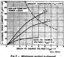
Fig.2 – Minimum output n-channel drain characteristics.
