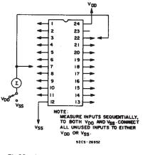
Fig.20 - Input leakage current test circuit.
