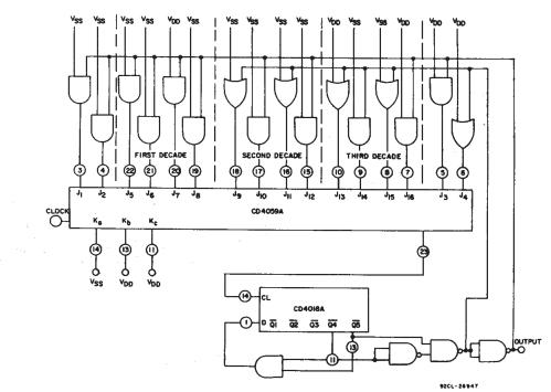
Fig. 15 - Dividing by any number from 88,003 to 103,999.
