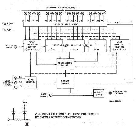
Fig.5 — Functional block diagram.
