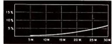
Fig. 3. Intermodulation distortion vs. power output.
